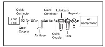
Figure 2. Installing your tool.
